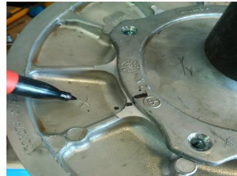
10) **Install new secondary spring.** You will notice that the spring has a tang on one end. This tang is to ensure the spring doesn't pivot on the aluminum end in the clutch which would cause wear. The roller assembly twists as it moves through the travel on the helix.
