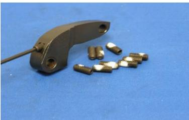
1) **Carefully** install the set screw into the threaded passage. Be careful, as the small M5 screws can easily be cross threaded. Wind the set screw all the way in until it is snug at bottom of threads.
